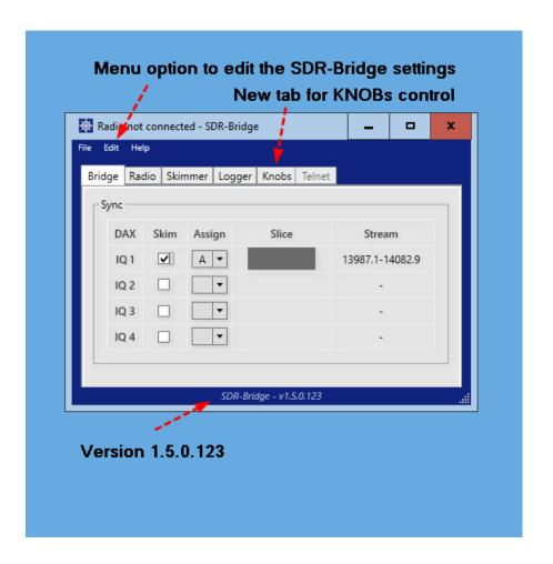
Note: The Telnet port in CW Skimmer must match the port shown here. For example IQ1 is 7310. See the CW Skimmer telnet port setup later in the document.
