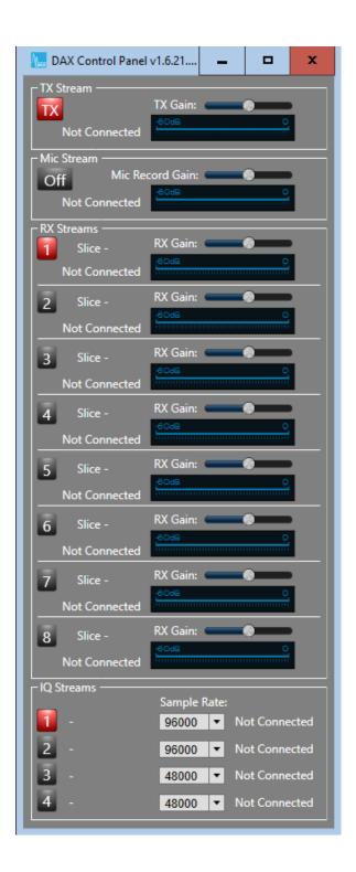
The only DAX setup needed for CW Skimmer is the IQ stream. To enable the DAXIQ channel, click the button for the channel you are using to ENABLE the channel, it should turn BLUE. Set the Sample rate to 96000. Note: in older versions of SSDR the rate is not persisted.
