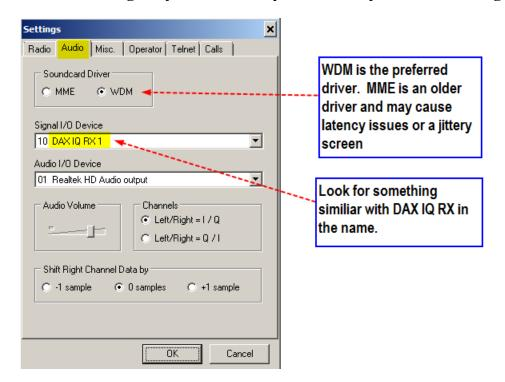
Note: Do NOT set the Audio I/O device to the same device as the Signal I/O device. This will cause issues. It should be set to one of your PC audio playback devices.
