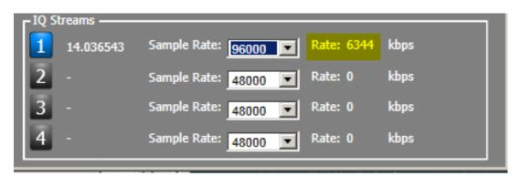
Starting in DAX V1.4 the RATE:value is replace with the word "Streaming" when running. You can see the rate by hovering the cursor.
